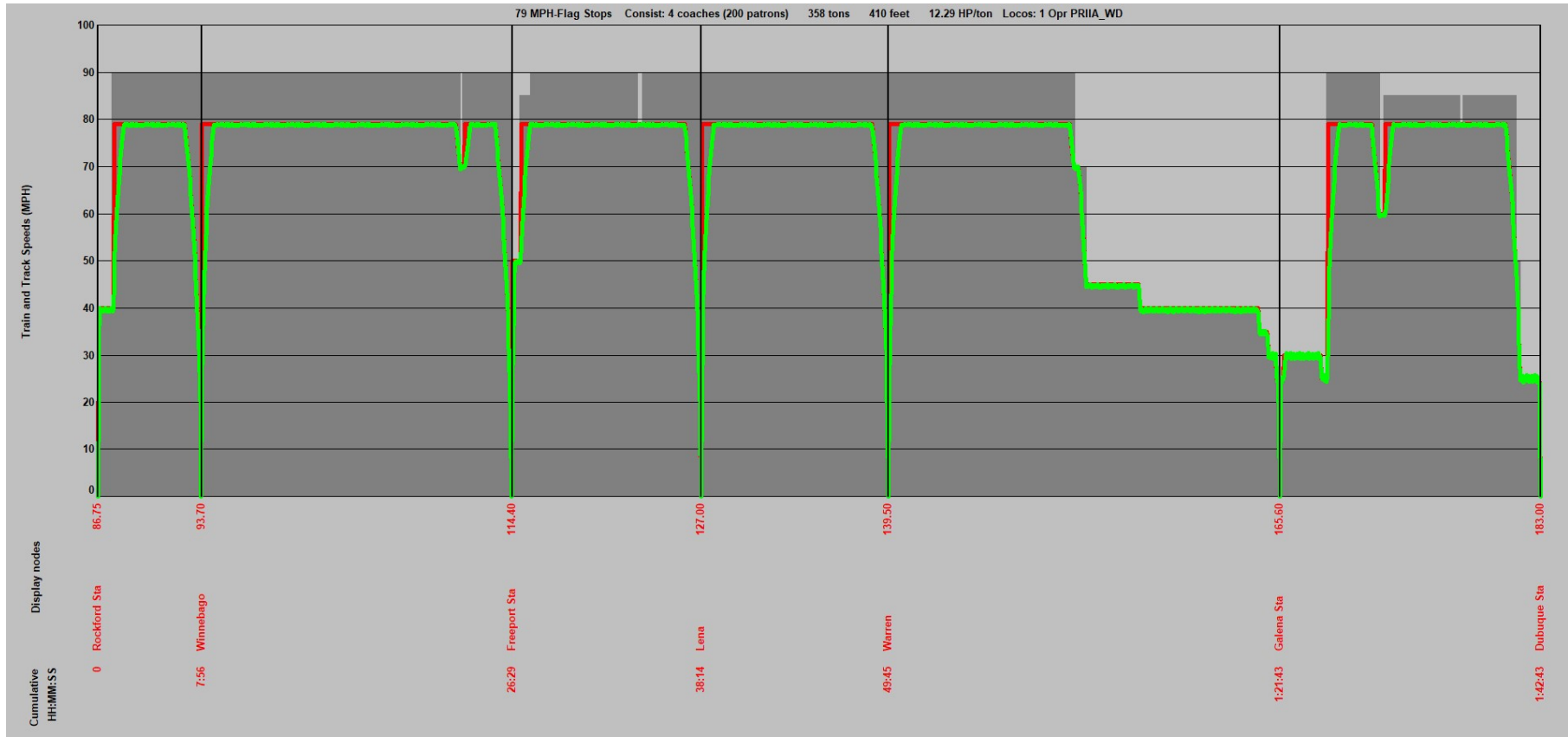
Pure Run Time Train Performance Calculator Output Chart – Primary and select secondary station stops at 79 MPH maximum speeds on CN
