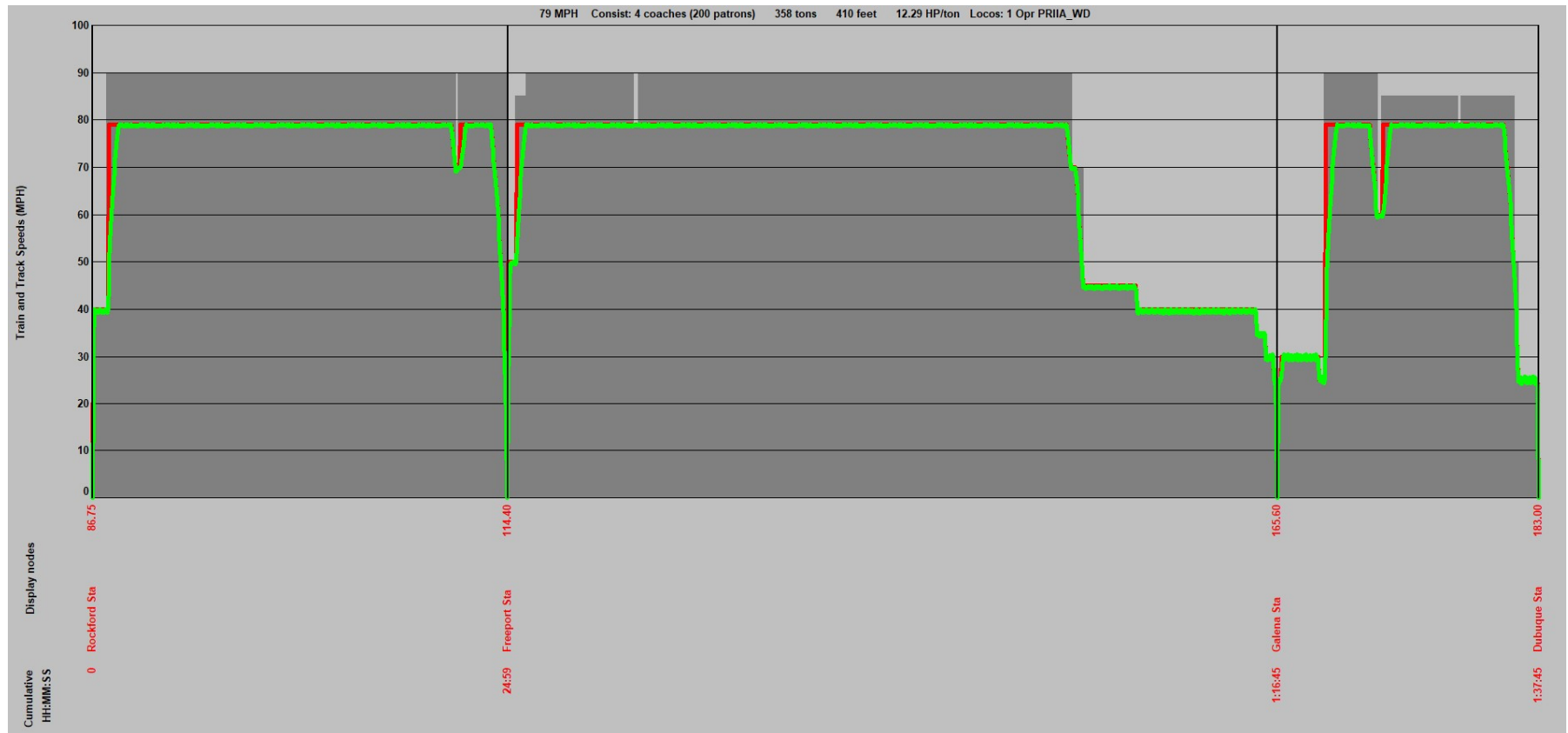
Pure Run Time Train Performance Calculator Output Chart – Primary station stops at 79 MPH maximum speeds on CN
